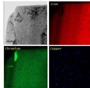
Figure 3. Characterisation data from 17-4PH aged for 24 hours at 560°C from TEM plus EDS (U. Huddersfield)
