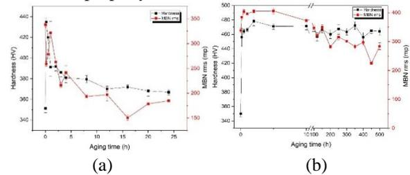
Figure 1. Variation of MBN and hardness with aging at (a) 560°C and (b) 482°C
