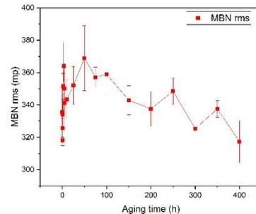
Figure 2. Variation of MBN in sample aged at 400°C (Correlate with precipitate evolution as per [4])
