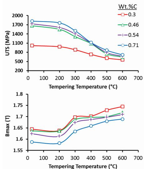
Figure 1. Variations of UTS and Bmax with tempering temperature for the samples with various carbon contents
