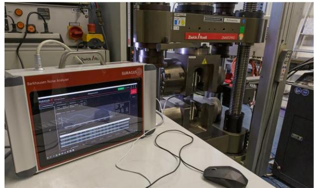
Figure 1. BNA equipment system during the testing on tensile machine
