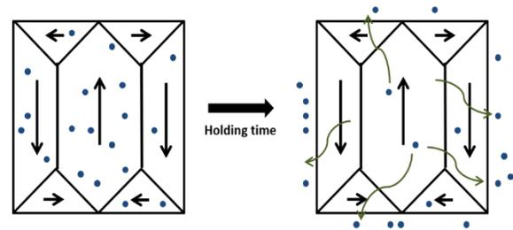
*Figure 1.* Schematic of a single grain (or magnetic object) indicating presence of magnetic domains and impurities within grains. Impurity migration towards grain boundaries, during temper embrittlement, can reduce interaction with magnetic domain structures.
