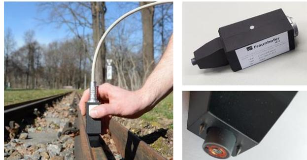
Figure 2. Current prototype device of Eddy Field BN sensor on IKTS.
