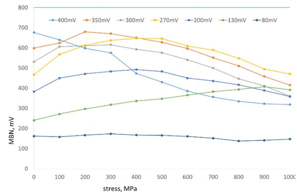
Figure 2. MBN versus tensile stresses for variable corrosion depths.
