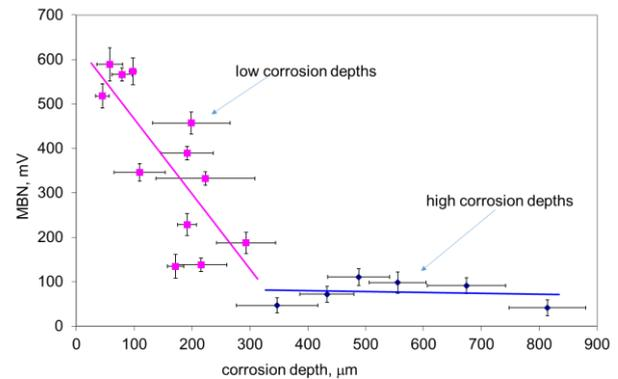
Figure 1. Corrosion depth versus MBN.
